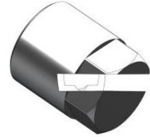
F0060003 Ø16x19; SW14; G1/4" Brass, Nickel-plated Sloped Slot 45°, broad
